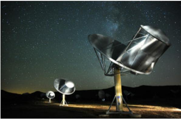
The Allen Array of radio telescopes is scanning the sky for artificial signals from extraterrestrial intelligences. Image courtesy of the SETI Institute.
